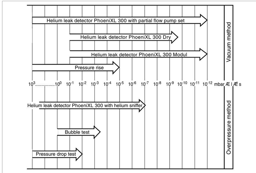
Overview of the leak rate detection ranges
