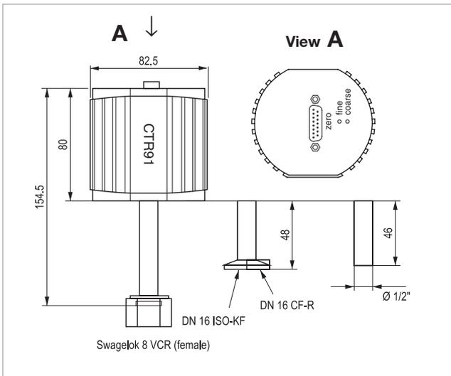
Dimensional drawing for the CERAVAC Transmitter CTR 91
