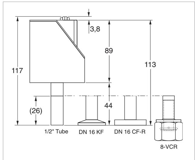
Dimensional drawing for the CERAVAC Transmitter CTR 100
