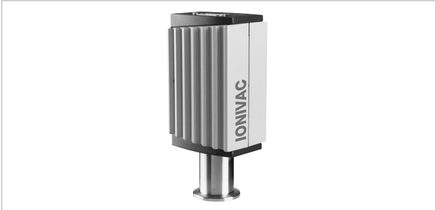
The ITR 90 is a optimized combination transmitter. The combination of a hot cathode ionisation sensor according to Bayard-Alpert and a Pirani sensor permits vacuum pressure measurements of nonignitable gases and gas mixtures in the pressure range from  $5 \times 10^{-10}$  to 1000 mbar.
