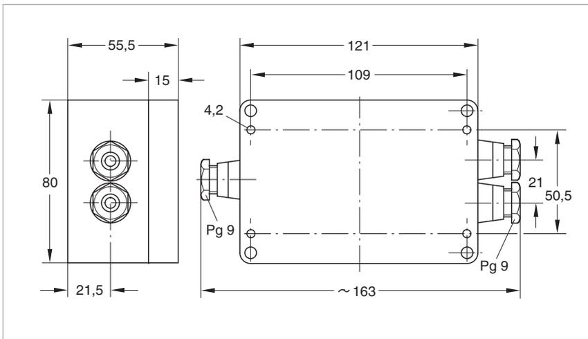
Dimensional drawing for the switching amplifier SV 110
