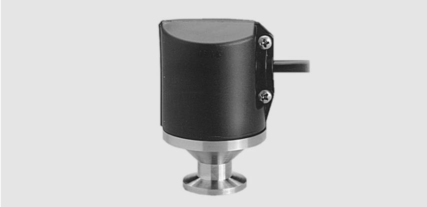
Switch indicating whether or not the pressure has reached the level of the atmospheric pressure after venting. Preset diaphragm pressure switch set to a trigger of 6 mbar (4 Torr) below atmospheric pressure.
