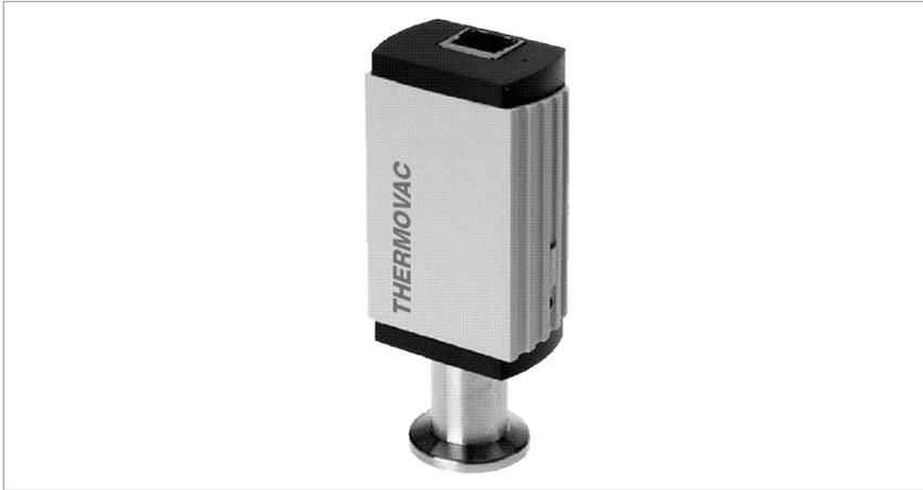
The Pirani Capacitance Diaphragm Gauge is the first vacuum gauge which combines ceramic capacitance diaphragm and thermal conductivity technologies. Unlike standard heat transfer technology, the Oerlikon Leybold Vacuum TTR 100 offers superior accuracy and gas-type-independent readings between 100 mbar and 1500 mbar.
