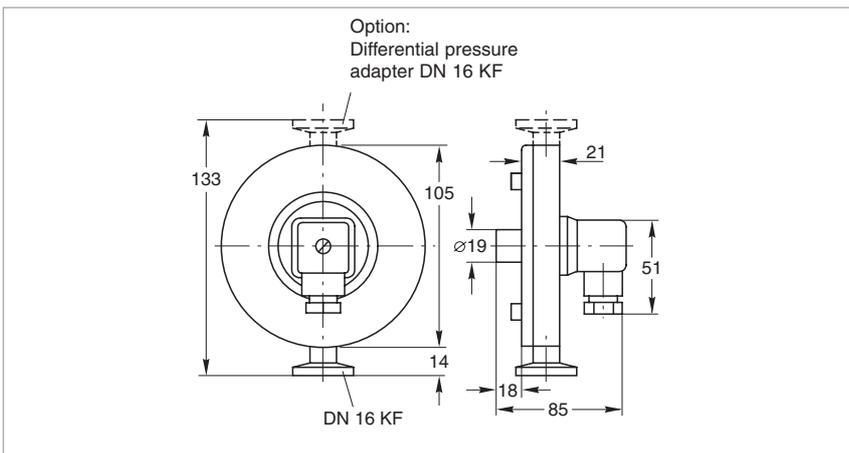
Dimensional drawing for the pressure switch PS 115
