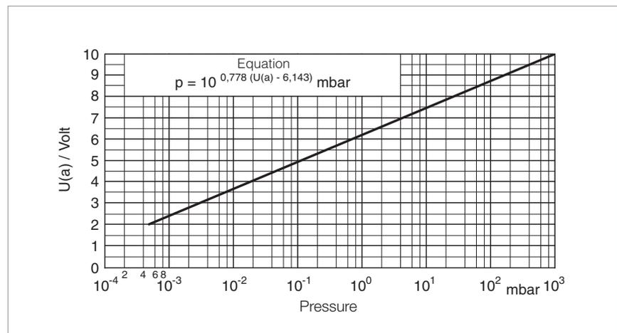
Characteristic of the THERMOVAC Transmitters
