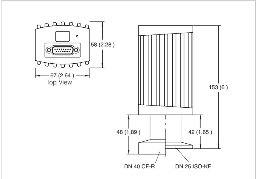
Dimensional drawing for the ITR 200; dimensions in brackets ( ) are in inch
