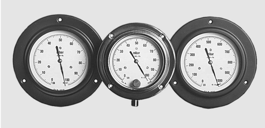
Rugged absolute pressure gauges for the pressure range from 1 to 1000 mbar (0.75 to 750 Torr).
