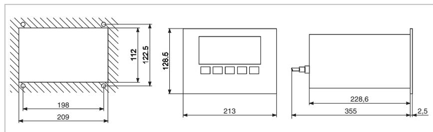
Front panel cut out (left) and dimensional drawing (right) for the IONIVAC IM 540
