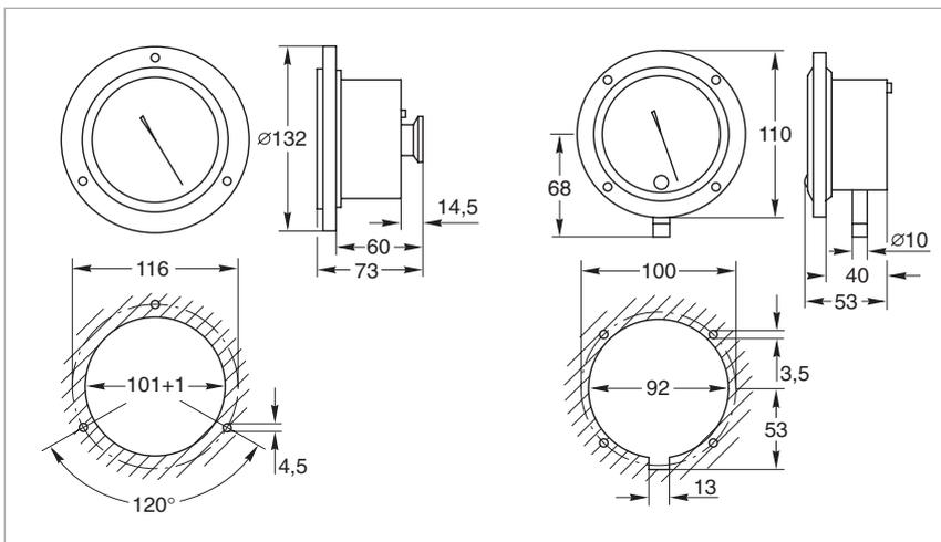
Dimensional drawings and panel cut-outs for the capsule vacuum gauges
