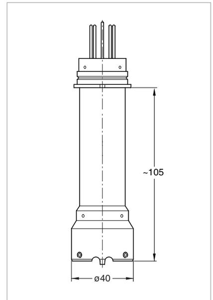
Dimensional drawing for the degassing extension
