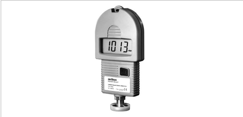
The THERMOVAC TM 90 is a simple handheld vacuum measuring instrument for occasional use. Its operation is based on the Pirani principle and covers a measurement range from  $1 \times 10^{-2}$  mbar to atmospheric pressure. It is delivered in a rugged plastic box.
