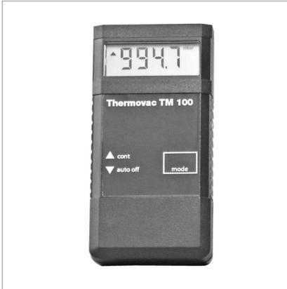
The handheld THERMOVAC TM 100 is capable of measuring pressures within the pressure range of  $5 \times 10^{-4}$  to 1200 mbar. By combining a piezo-resistive pressure sensor for the upper and a Pirani sensor for the lower pressure range, the measurements made by the THERMOVAC TM 100 are independent of the type of gas above pressures of 15 mbar. Especially noteworthy is the exceptionally long battery life.
