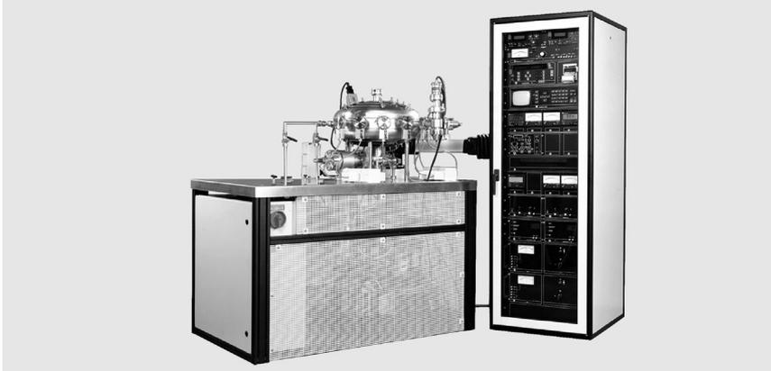
Calibration of vacuum gauges in the pressure range from  $10^{-9}$  to 1000 mbar ( $10^{-9}$  to 750 Torr) as DKD or factory calibration.
