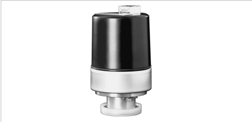
The PENNINGVAC transmitter combines the cold cathode ionization principle with the Pirani principle. This allows for complete coverage of the pressure range from  $5 \times 10^{-9}$  mbar to atmospheric pressure by a single transmitter. The cold cathode system is ignited directly through switching on the internal high-voltage at the optimum ignition pressure.
