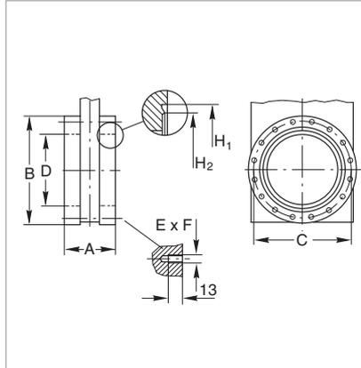
Connection dimension for CF flanges (UHV Gate Valves)
