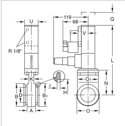
Dimensional drawing for the miniature UHV gate valves; electropneumatically operated, ISO-KF flange
