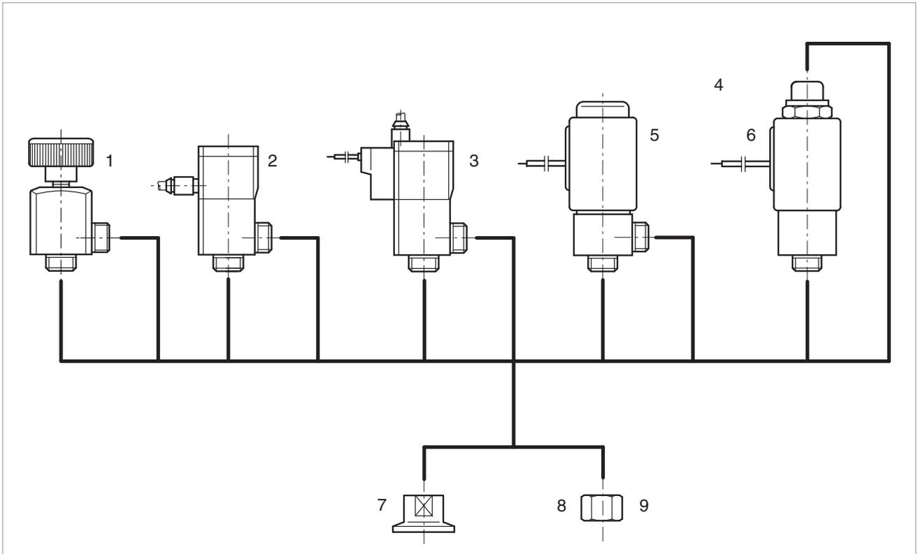
Oerlikon Leybold Vacuum small valves **micro** are available with any of four drive systems, two types of body and three adapters.
