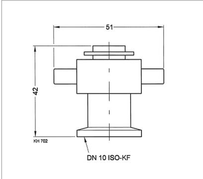
Dimensional drawing for the venting valve, manually operated
