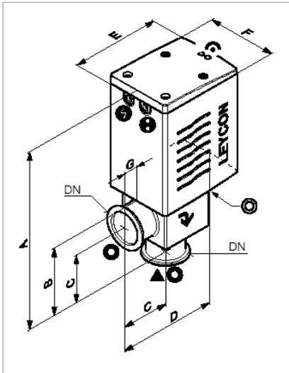
Dimensional drawing for the bellows-sealed right-angle valves
