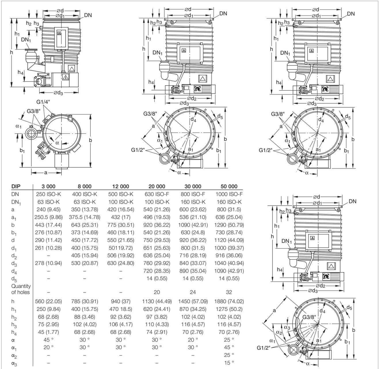
Dimensional drawing for the DIP 3000 [top left], DIP 8000 to DIP 20 000 [top middle], DIP 30 000 [top right] and DIP 50 000 [bottom right]; Dimensions in brackets ( ) are in inch
