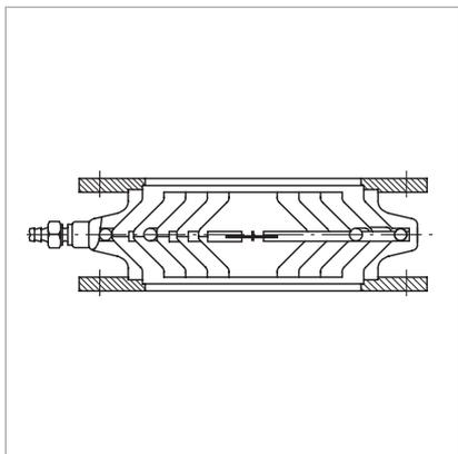
The cooling inserts of the astrotorus baffles are made of copper, whereas the housing and the connection flange are made of standard steel.
