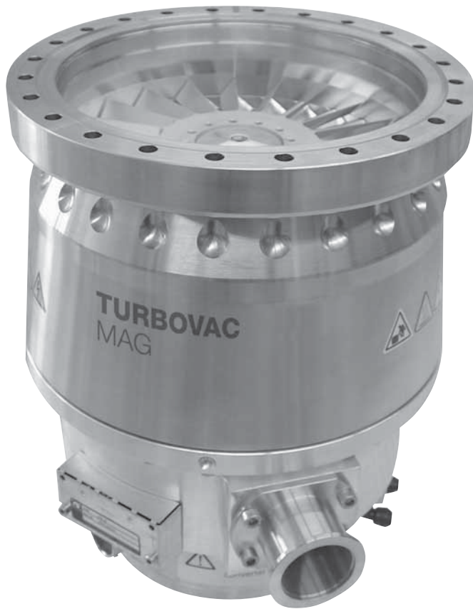
MAG W 1300 C turbomolecular pump with magnetic rotor suspension and compound stage
