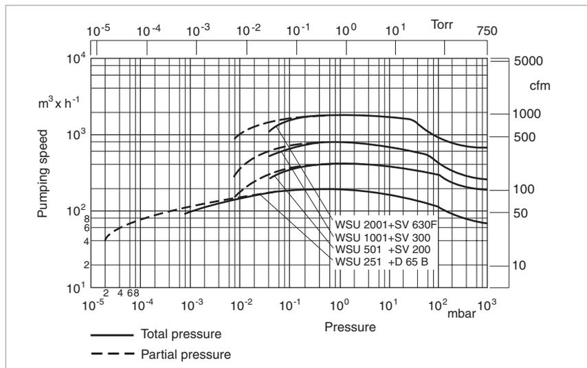
Pumping speed of the RUVAC WS/WSU, 50 Hz
