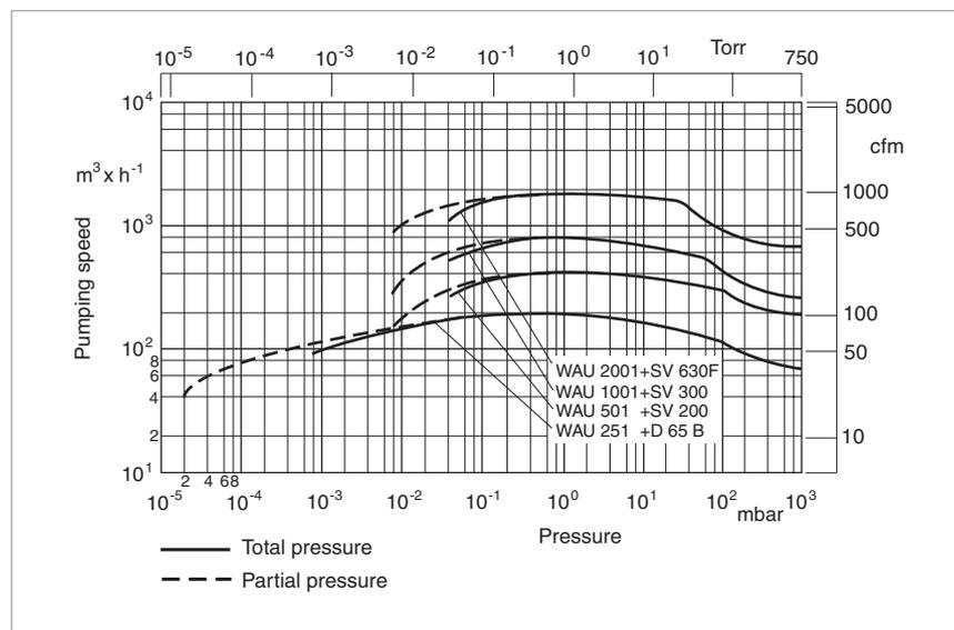
Pumping speed of the RUVAC WA/WAU, 50 Hz
